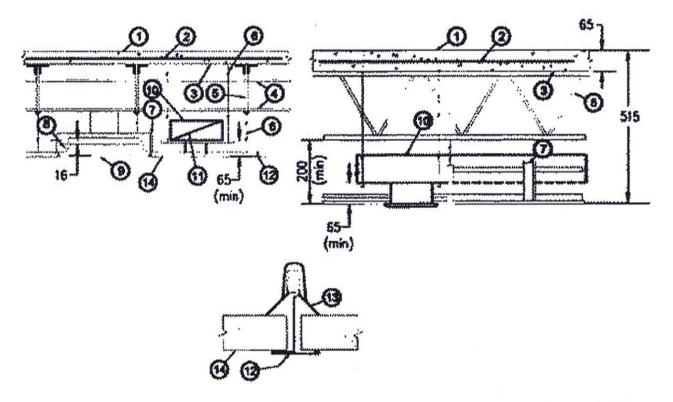
**Beam** — W8x24, min size. As alternate to steel beam, **Joist girders** (Not shown) — 20 in. min depth and 13 lb/lin ft min weight.
